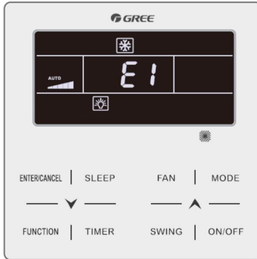
Power-on High-pressure Protection Fault Interface
